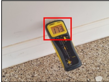
Higher than normal moisture reading present
