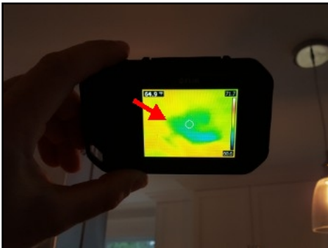
Evidence of poor insulation at kitchen
