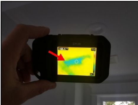
Evidence of poor insulation at master bath
