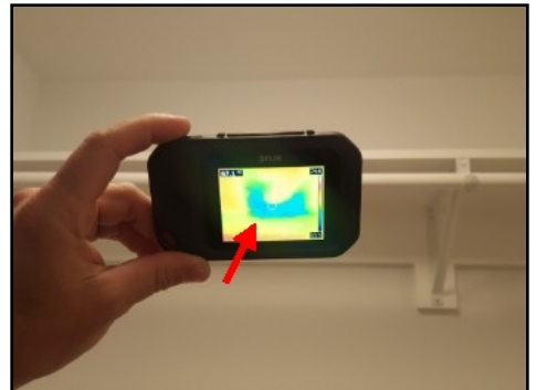
Evidence of poor insulation at master closet
