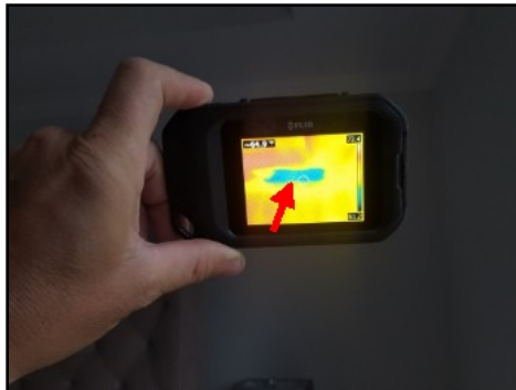
Evidence of poor insulation at master bedroom
